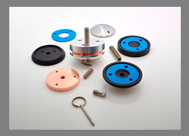
The robust-yet-elegant MPOD is comprised of multiple machined aircraft-aluminum and tungsten-steel parts that, when assembled, form a vertical stack. A solid pure-copper substrate center section is sandwiched by a top and bottom layer of ISODAMP -- a thermoplastic material that, when compressed against the copper substrate, facilitates the constrained layer damping function and dissipates unwanted energy virtually immediately.
